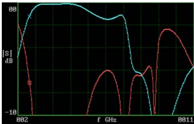
Fig. 7: Frequency behavior of a branch line coupler with decreased characteristic impedance, Z_1=35.5\Omega, Z_2=80\Omega, Z_3=70\Omega, Z_4=40\Omega, \theta_1=45^\circ, \theta_2=45^\circ, \theta_3=30^\circ, \theta_4=10^\circ electrical length
